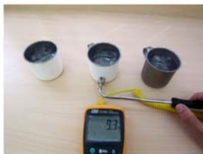
塗覆一般隔熱塗料，鋼杯外側溫度9.3°C Apply common thermal insulation coating. The temperature of outside steel cup is 9.3°C
