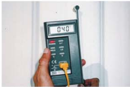
施作COAT PC200後，屋頂板表面溫度 Surface temperature of the roof deck after application of COAT PC200
