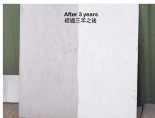
圖片中右半部的COAT PC200表面經過COAT PT301處理，三年之後仍常保如新 After three years, the COAT PC200 surface with COAT PT301 on the right side remains clean.
