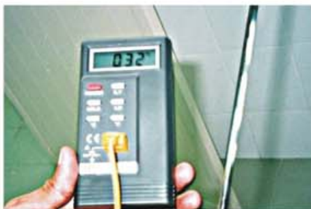
施作COAT PC200後的室內溫度 Indoor temperature after application of COAT PC200
