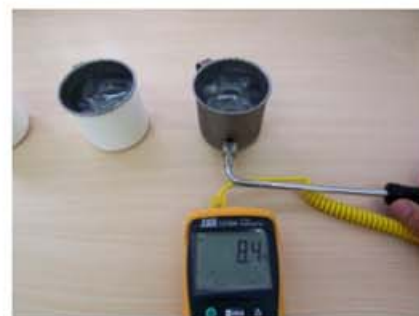
沒有塗覆隔熱塗料，鋼杯外側溫度8.4°C Without any coating, the temperature of outside steel cup is 8.4°C
