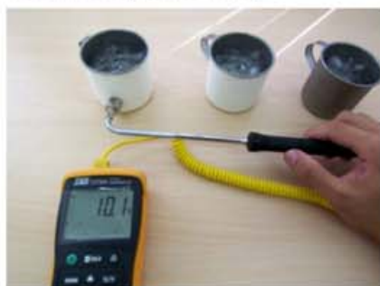
塗覆COAT PC200，鋼杯外側溫度10.1°C Apply COAT PC200 coating. The temperature of outside steel cup is 10.1°C
